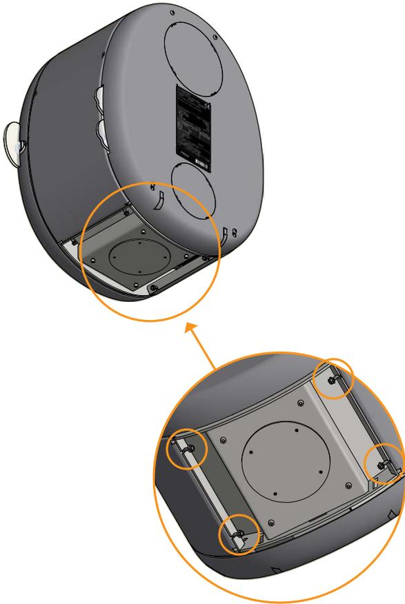
Remove the screws from the rear plate.
