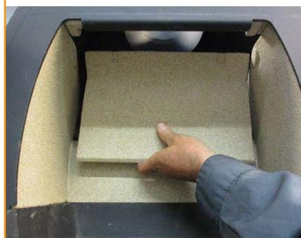
Push the plate upwards so that it rests on the front plate
