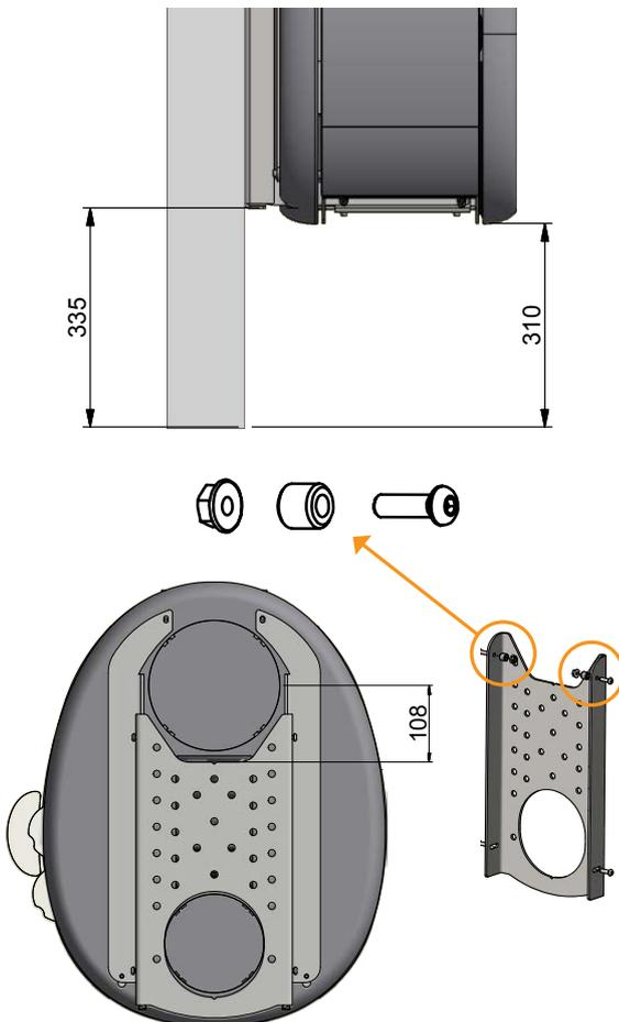
Remove the slits - use a drilling machine and nippers
