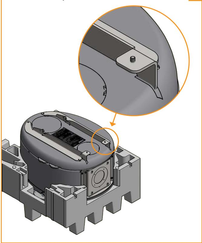
Adjust the stove so that the doors has the correct slope 11
