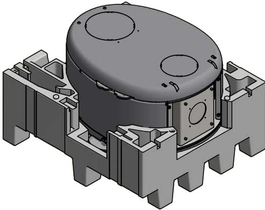
Dismount the rear plate by removing the four screws. Place the rear plate on an even surface
