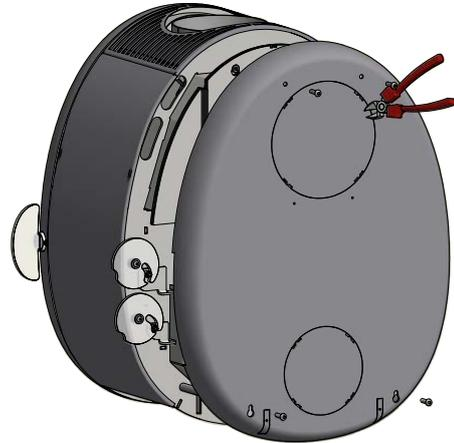
Using cutting pliers, cut off the cover plate from the heat shield at its securing points
