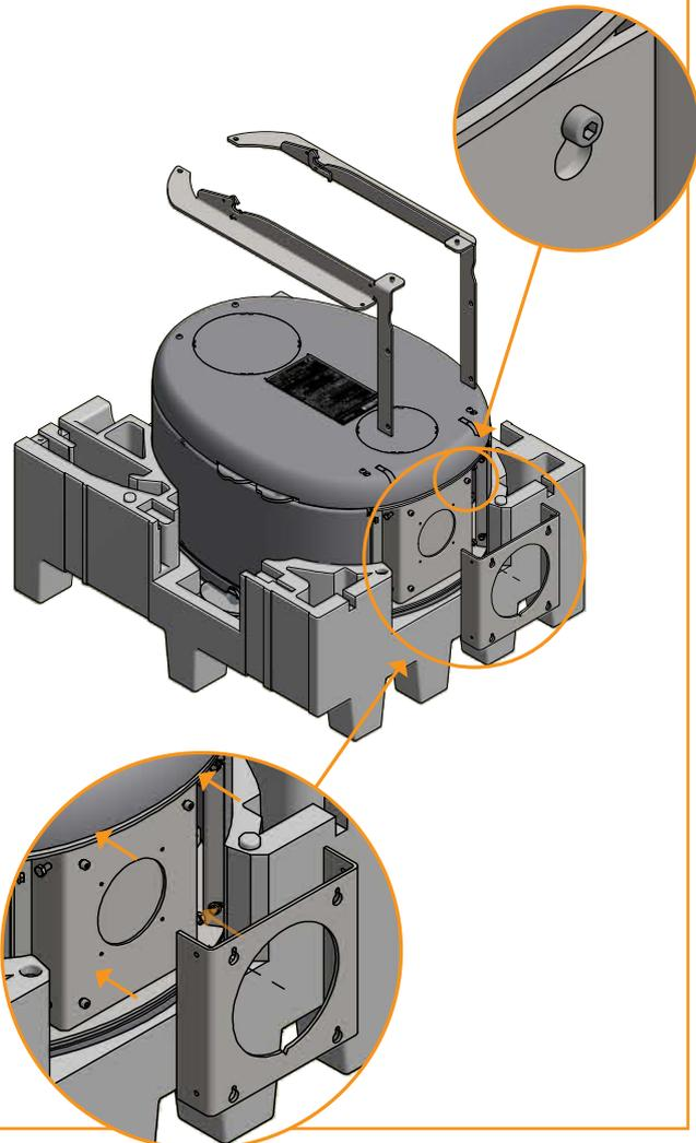
Mount the four screws loosely in the rear plate again, now with the wall fitting in between.
